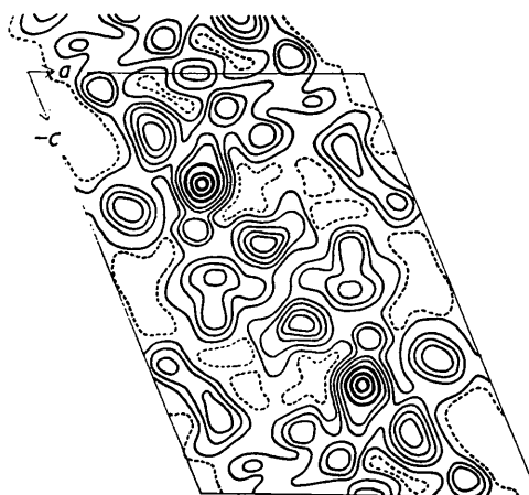
Fig. 5. Electron density projected along b on the ac plane. The contours are drawn as for Fig. 3.
